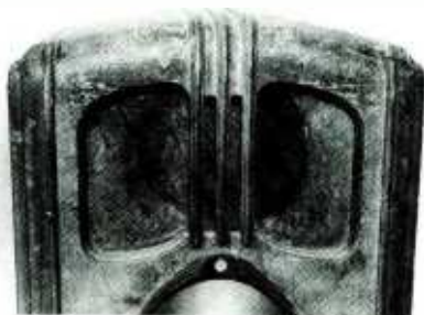
This close-up of the cabinet top shows the ravages of a furnace explosion. By next month, I hope to have cabinet looking beautiful again.
