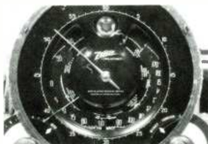
Close-up taken just before installation of the dial glass shows the action of the shutters. The broadcast-band shutter set is being swung out of the way to reveal short-wave band calibrations.
