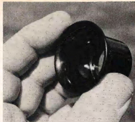
A x2 magnifier is handy for inspecting valve filaments and cathodes. The cathode in a good valve will be coated with a whitish compound.
