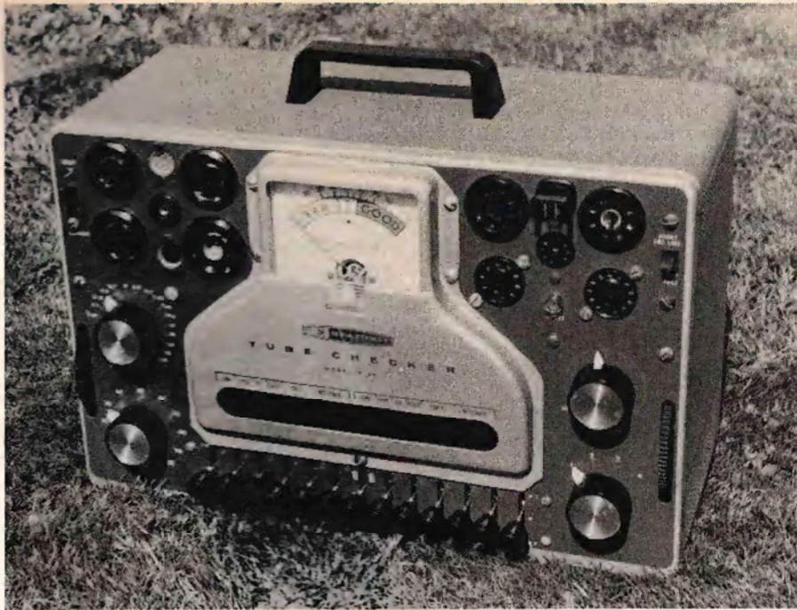
Although not essential, a valve tester eliminates a lot of uncertainty when checking valves. This is the author's Heathkit Tube Checker. Valves can also be tested by direct substitution in a known good chassis.
