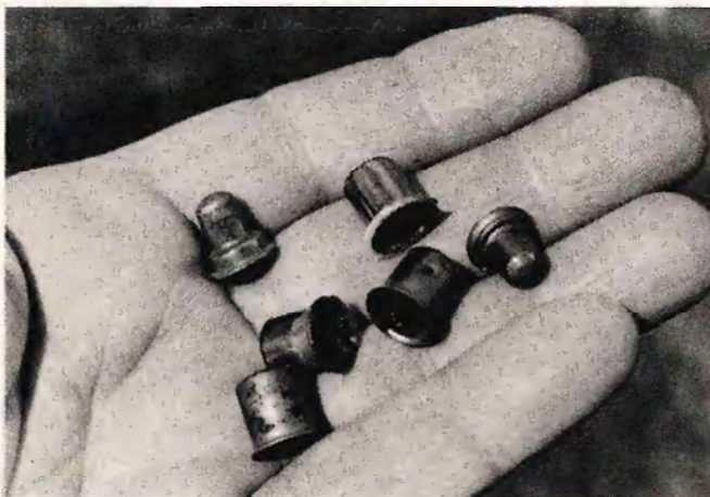
Loose or detached top caps can be a problem with old valves. The valve can be saved by carefully resoldering the cap and then re-gluing with "Super Glue".
