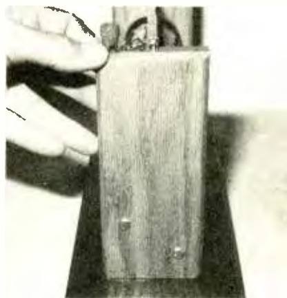
This is a close up of how the oak supports are tied to the panel.
