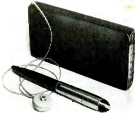
Whole receiver is no taller than a standard fountain pen.
