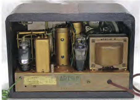
The rear view highlights the two substantial metal screens fitted to the 6U7G and 6B8G valves. Note the top-cap grid leads for the first three valves. This was common in pre-war receivers to minimise the effects of stray capacitance.
