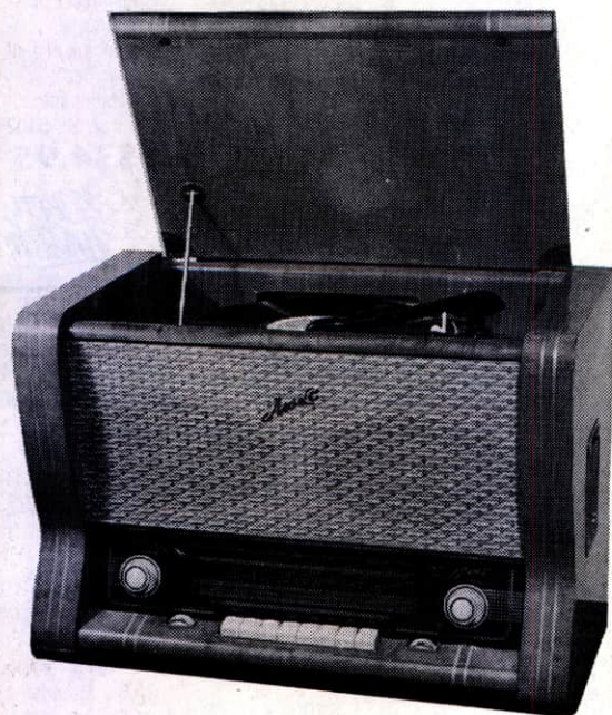
Right: In its distinctive tabletop cabinet, the Russian radio/record player would stand out in any collection. There are a total of six receiving bands, including an FM band centred on 67MHz.
