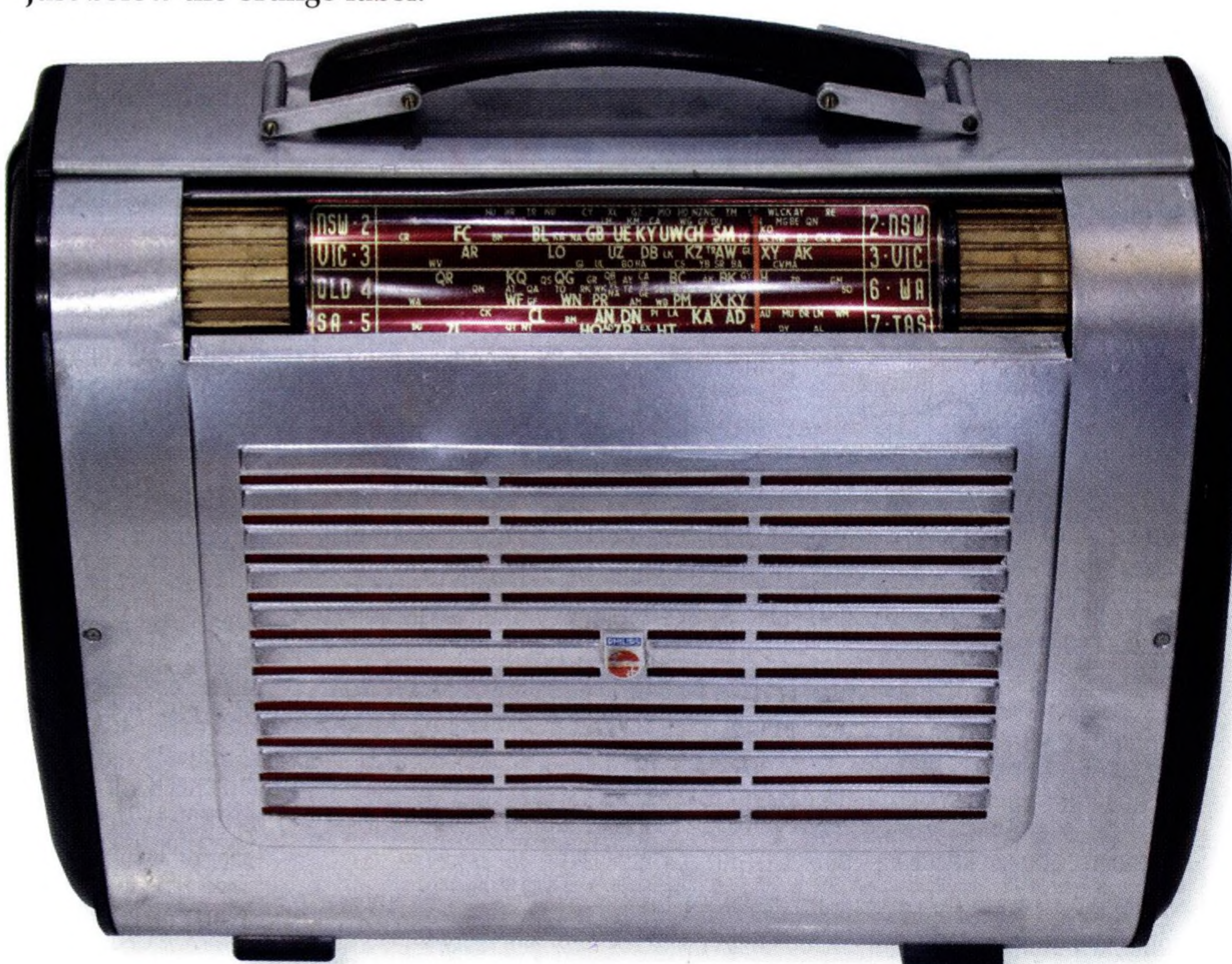
Not all of these portables made by Philips were equipped for mains operation as can be seen by the add-on section above involving the 6V4 full-wave rectifier just below the orange label.
