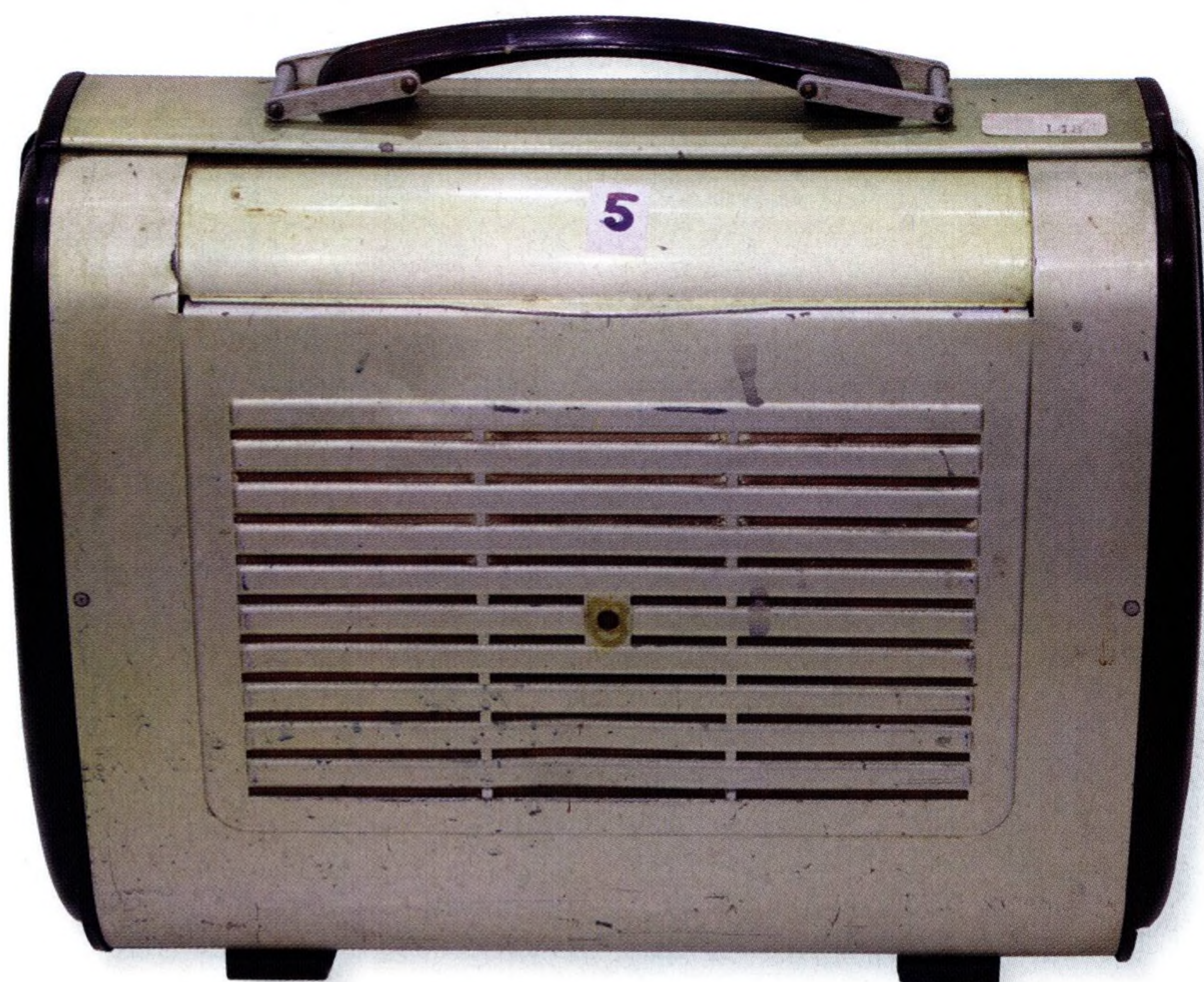
The unrestored aluminium case with the dial shutter closed and badge removed. The radio does not have an on/off switch, but instead is turned on by opening the shutter.
