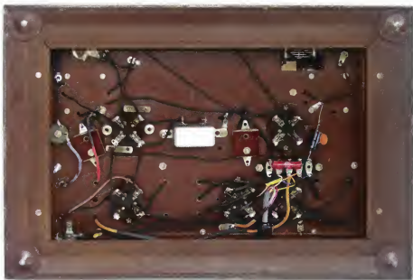
This is the view underneath the chassis. The set is logically laid out and the various stages on top of the chassis are separated by metal shields to prevent interaction between them.
