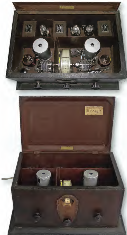
The lid of the SW5's cabinet is hinged at the back, so that it can be opened to change the plug-in coils for different bands. There are just three front-panel controls: regeneration (left), tuning (centre) and antenna peaking (right).
