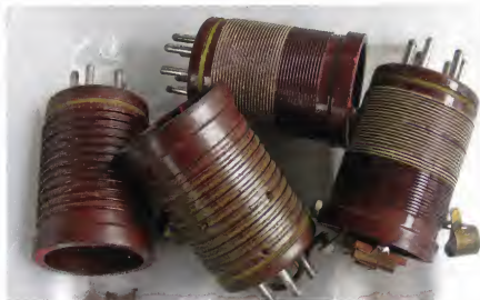
This photo shows just some of the plug-in coils used with the receiver. Four pairs of coils were supplied as standard and additional coils could also be purchased.
