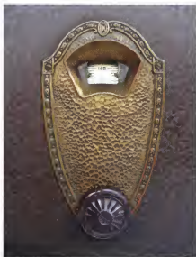
A simple numbered dial-scale was used in the SW5 receiver, so users normally kept a list showing where various stations appeared.
