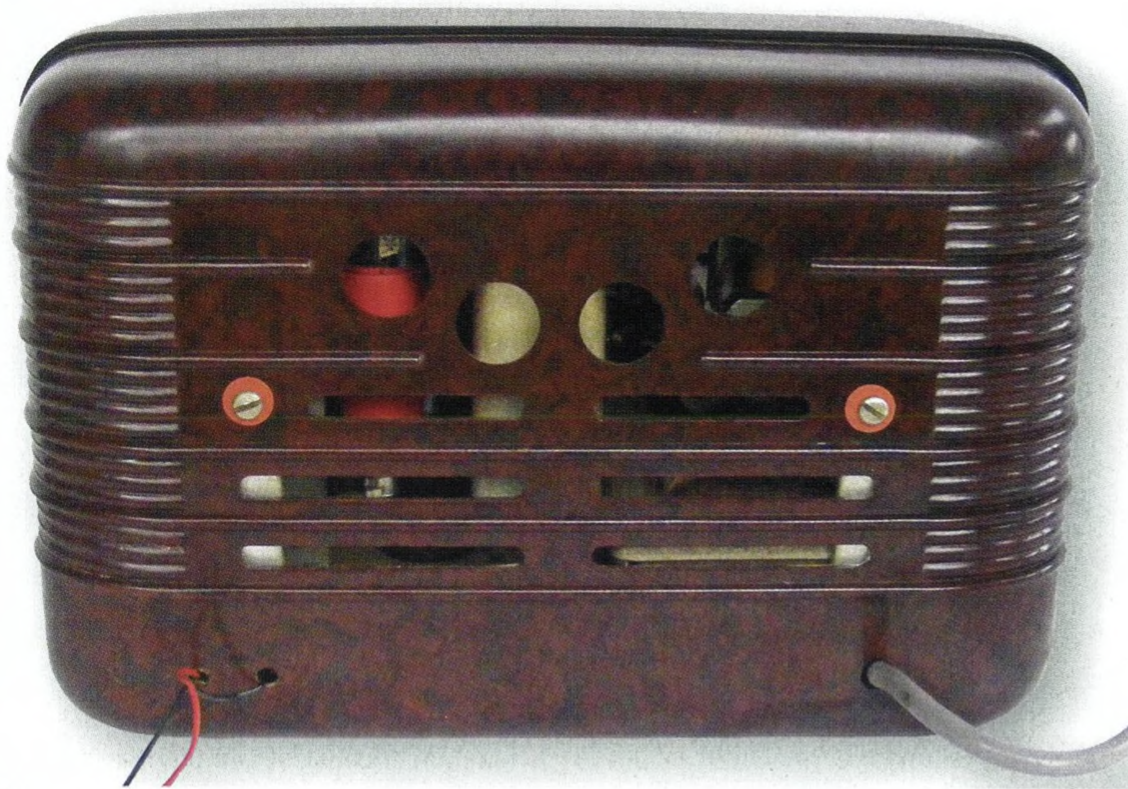
The rear section of the cabinet has four large “finger holes” so that the set can be easily picked up and carried. Undoing the two screws allows the rear section to be removed and provides good access to most parts with the chassis in-situ.
