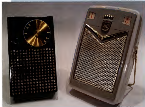
Shown at right in the above photo, Grundig's 1958 Taschen-Transistor-Boy was much larger than Regency's shirt-pocket size TR1 receiver (left).
