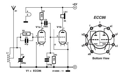
impedance of 2 k $\Omega$ . A 500-pF capacitor between the two stages ensures that RF signals will not be further amplified. Otherwise the valve might easily recall its original intended use and start oscillating in the short-wave range. A ferrite rod with a diameter of 10 mm and a length of 100 mm, with a winding of 50 turns of enamelled copper wire, serves as the aerial.
