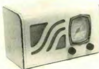
The 1939 Philco set shown here was one of the last wood-cabinet table models in the line. Note the large tuning dial with rotating pointer.
