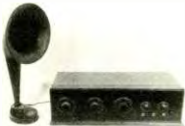
The three-dial battery-operated TRF was common in the 1920's. The one shown in this photo is a Neutrodyne and was originally built from a kit.
