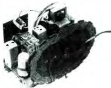
This view of the Emerson's chassis shows the loop antenna, the "GT"-type tubes, and its square-topped IF-transformer cans.
