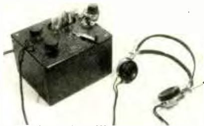
The RCA Radiola III is good example of a typical regenerative receiver. Its two-tube circuit made loudspeaker operation possible, especially on strong local signals.
