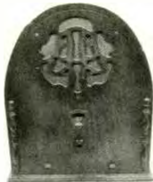
The Cathedral-style Gloritone screen-grid set represents the transitional period of radio-receiver development. Note that the tuning dial is viewed through a tiny window.
