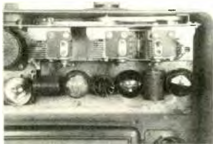
A "straight-down" view of an open Model 42 cabinet shows belts and pulleys linking the tuning condensers for single-control operation. The corner of the separate power-supply box is seen at the lower left of the photo.
