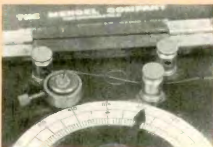
A crystal detector consisted of a fine wire (the "cat's whisker") in contact with a fragment of galena (lead ore). The version shown does not have the usual swivel-arm mount for the wire.
