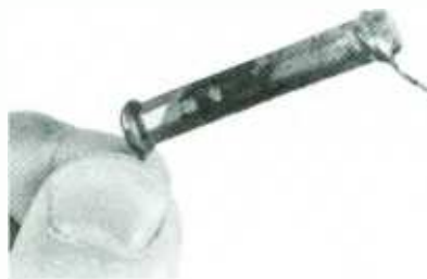
The overheated burned resistor was replaced with a new one of the proper value. Finding problems like that up front eases troubleshooting later.
