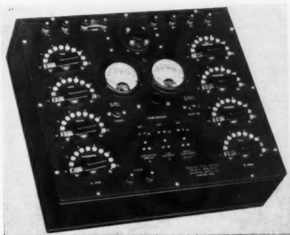
Fig. 4—Bridge circuit for vacuum tube measurements
