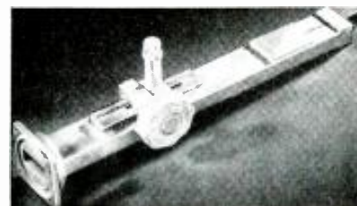
Fig. 12—A tuned load for 8200-12400 mc.
