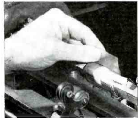
Putting insulating fiber between windings evens up the surface and provides insulation.
