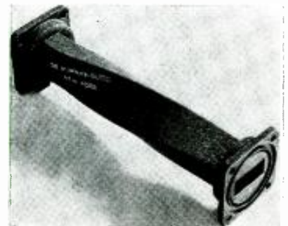
Fig. 16—This section changes polarization. precision-cut so as to absorb any leakage power and cause a minimum of reflection at the junction.
