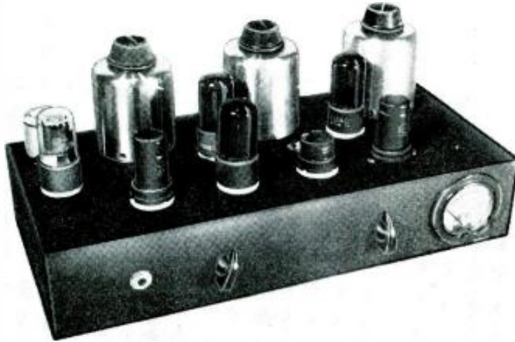
Front view of the phase-modulated exciter. The signal of a low-frequency crystal is multiplied eight times to hit 80 meters.
