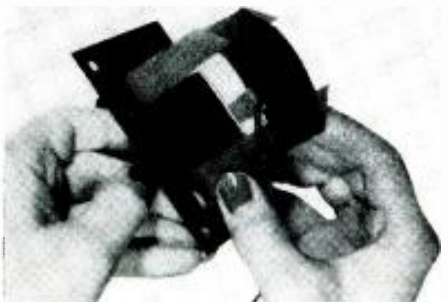
Last job of all is inserting laminations. This is not hard to do if all the dimensions are correct.
