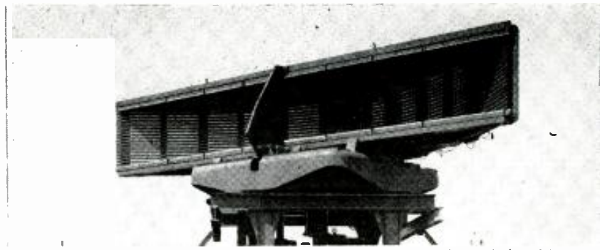
Close-up of the rotating "cheese" antenna, built of strips to reduce wind resistance.
