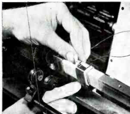
turn through and pull loop ends tight. If winding ends midway, use loop as above, wind a few turns over it and slip end turn through.
