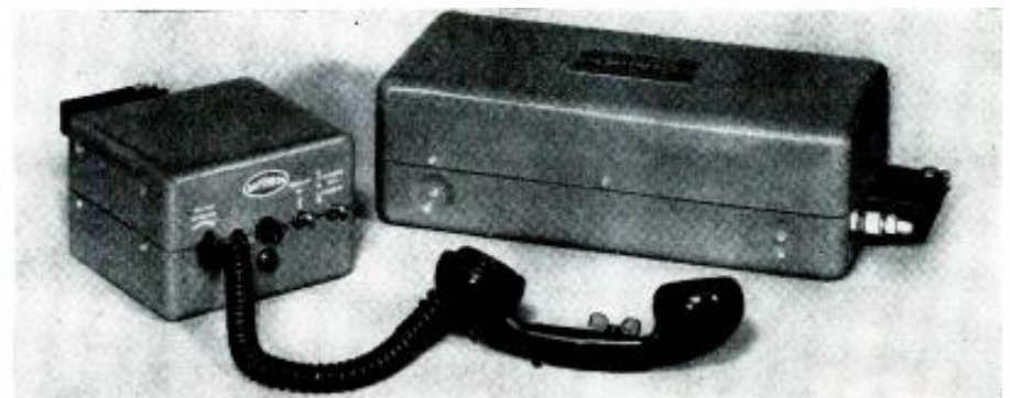
Raytheon transmitter-receiver (right) and control box (left) show compactness of equipment.
