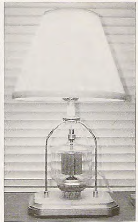
Photo G. Lamp made from a 3-500Z.
