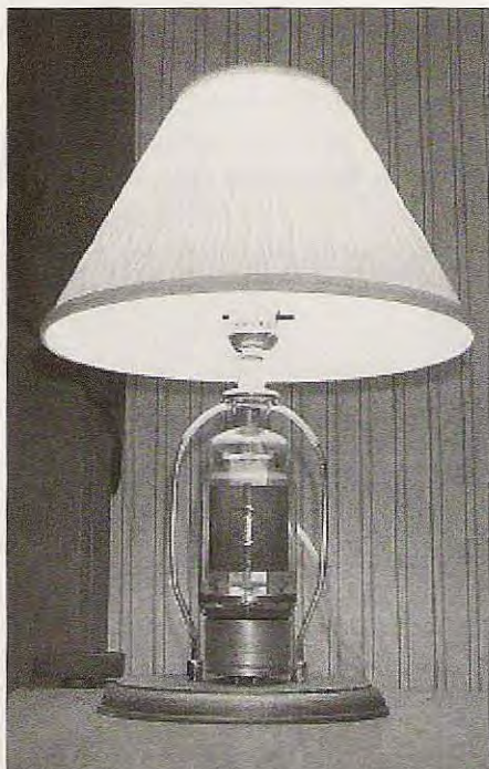
Photo A. My first lamp — and my favorite — is made from an 813 tube.
