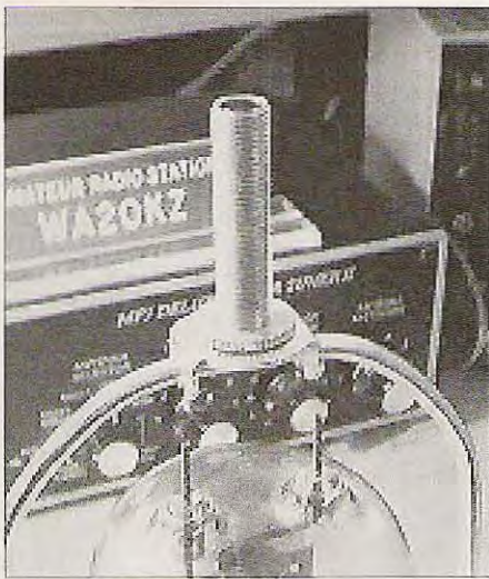
Photo D. Solder the nut with the threaded pipe to the top of the harp.
