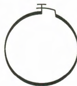
Figure 2. Hertz's receiving antenna - a Knochenhaur Coil.
