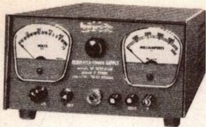
(Left) The Kepco Type SC, the company's first 'transistorised' power supply. (Centre) The Kepco Type KM, a high power supply using a magnetic-amplifier control system. (Right) The Kepco Model 700, a vacuum tube supply delivering 0-350V DC at up to 750mA.
