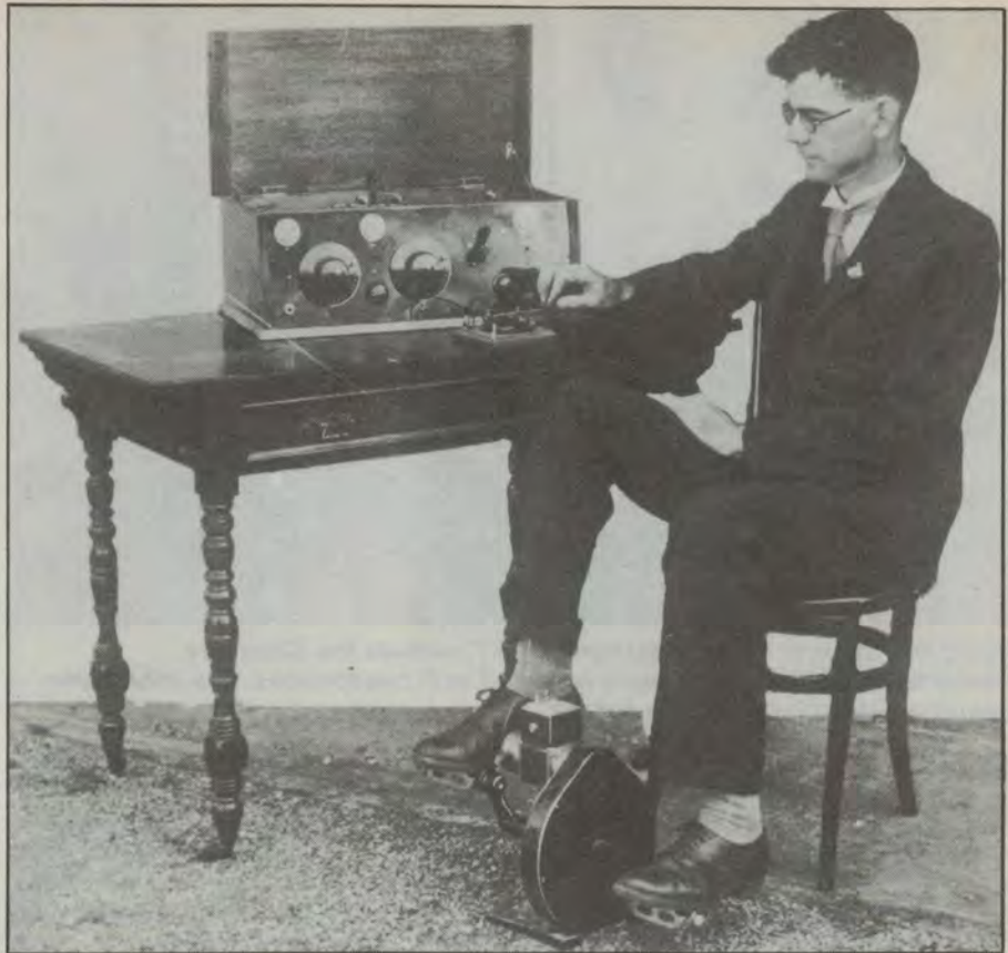
Pedal radio inventor Alfred Traeger shown demonstrating one of his remote station sets in 1929. Note the morse key and pedal generator.
