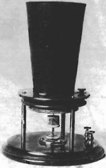
FIG. 2—THE LIQUID TELEPHONE. It was over this device that the historic words "Mr. Watson, come here, I want you!" were spoken on March 10, 1876.
