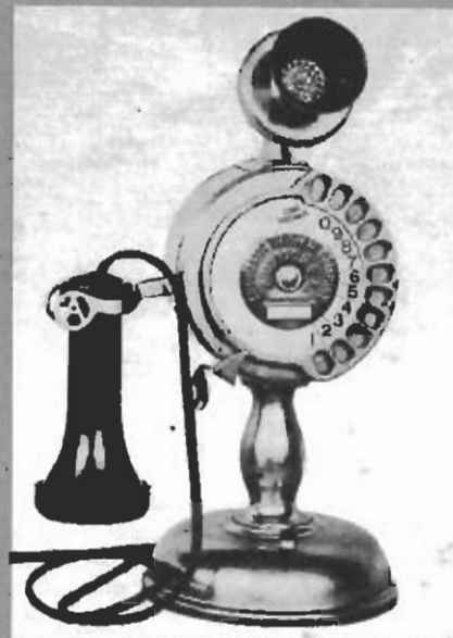
FIG. 5—A STROWGER automatic telephone (dial-type). The invention of this phone eliminated the need for manual switching.
