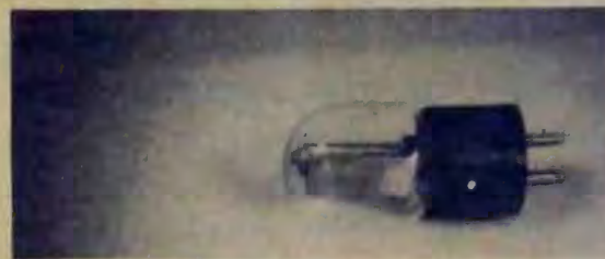
Fig. 9 Another early type of phototube.
