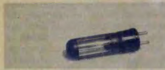
Fig. 10 A phototube with a "window" envelope.
