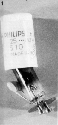
Figure 1. Photograph of a partly dismantled fluorescent-lamp glow-starter. Note the suppression capacitor.
