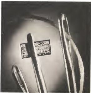
Fig. 16 Integrated circuit chip compared with ordinary sewing needle, the chip being 1.5 × 3mm
