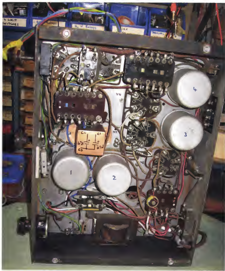
The underside of the chassis is quite neat. The silver cans marked 1-4 contain the coupling transformers, while the two copper boxes on the underside and top (left of the dial) of the chassis contain electrolytic capacitors.
