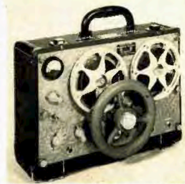
Fig. 15. Spring driven motor and battery powered amplifier are used in this Amplifier Corporation of America portable.
