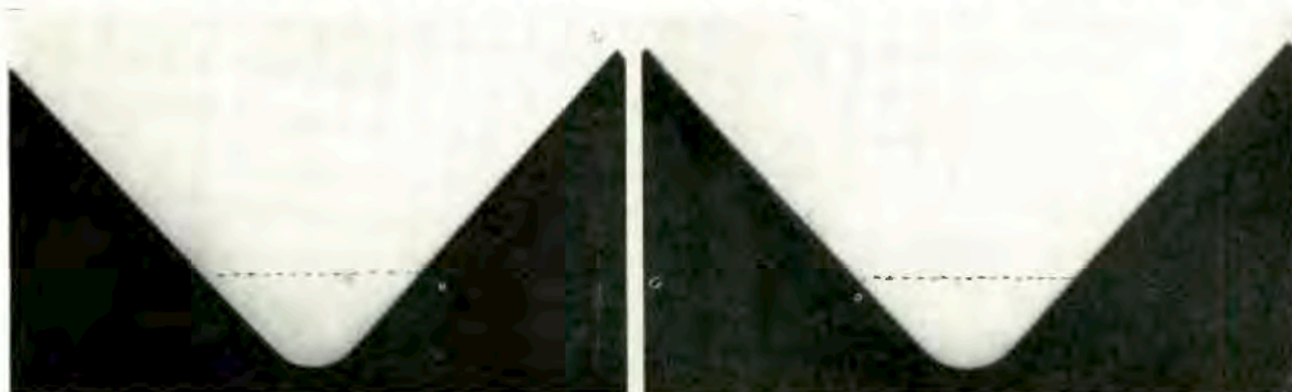
Fig. 11 (left) & 12 (right). Contact prints of shadowgraphed two-faceted styli. The dotted line indicates the functional portion for 100 lines per inch and consequently the portion below this line will be the resultant groove shape. Deviation from "ideal" shape lies in the fact that in Fig. 11 the radius does not blend perfectly with the angle on one side.
