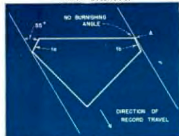
Fig. 3a. Same stylus cross-section in groove whose slope is 30°. Burnishing facet 1a forms angle of 55° with adjacent wall. Facet 1b cannot burnish with groove slope in excess of its basic angle. In fact, the edge formed by the meeting of cutting face and burnishing facet (A) will tear the adjacent groove wall.
