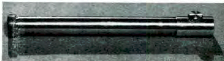
Transducer probe for use in air. Details of the interior of the crystal mounting are shown in Fig. 3.
