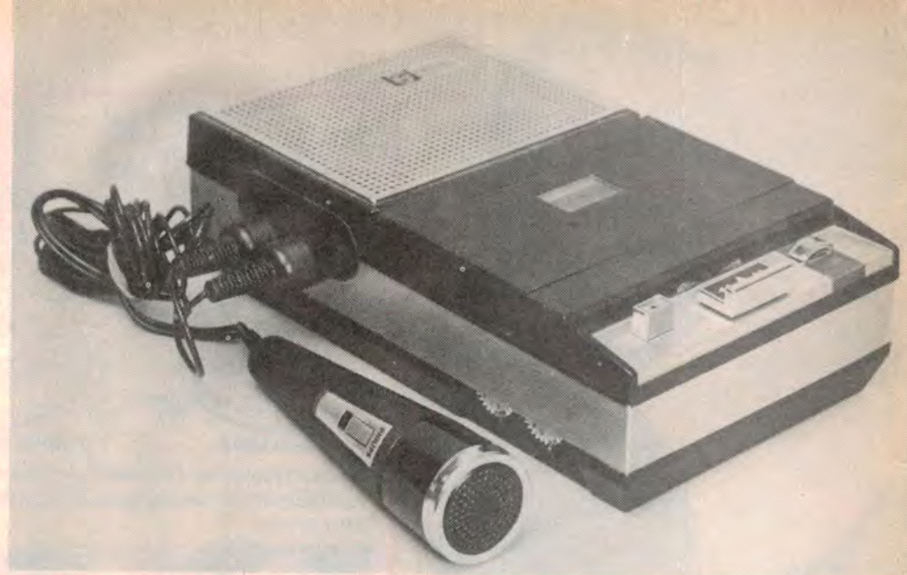
The Philips EL-3302 battery-powered portable, which did much to establish the compact cassette format in Australia.
