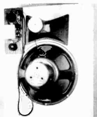
Fig. 8. Baffle with two-cell Racon horn and 15" Jensen cone and dividing network for 1,200-cps crossover frequency.
