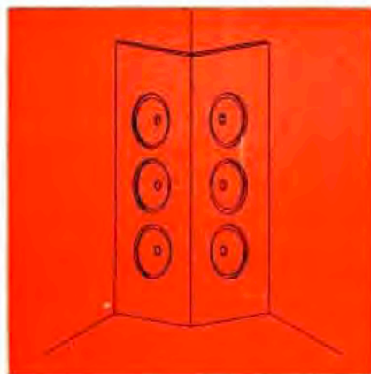
Fig. 1. Mounting a number of ordinary cones on two sides of an obtuse structure for corner use is one solution to the necessity for moving more air.
