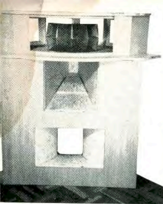
Fig. 3. Front view of the new speaker during construction, showing the speaker well and the TV tube enclosure.
