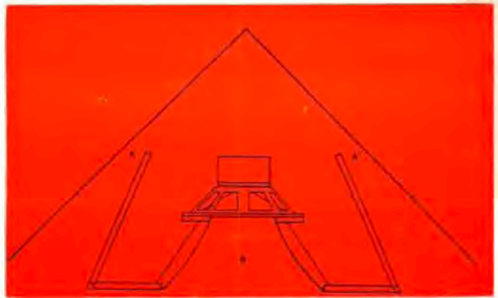
Fig. 2. Plan view of the new corner speaker design, showing vents at either side between the cabinet and the wall, and the horn loading provided by the wall and the cabinet sides.
