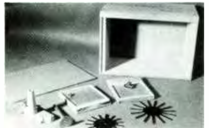
This is the preliminary stage in the construction of Dan Damrow's Crosley 50 replica. The fabricated parts for the coils and "book" condenser are in the foreground.
