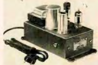
Fig. 4. Another self-powered preamplifier is the Pickering, Model 230H, with vibration-reducing rubber grommets for mounting.
