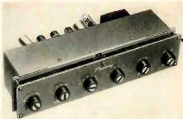
Fig. 6. Typical of complete control units is the Pickering Model 410 Audio Input System, which has volume and tone controls in addition to preamplifier.
