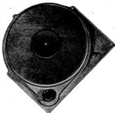
Argonne Model AR-340 is a single-speed 33 \frac{1}{3} rpm turntable with hysteresis motor, has die-cast aluminum turntable, comes with a rubber disc mat.
