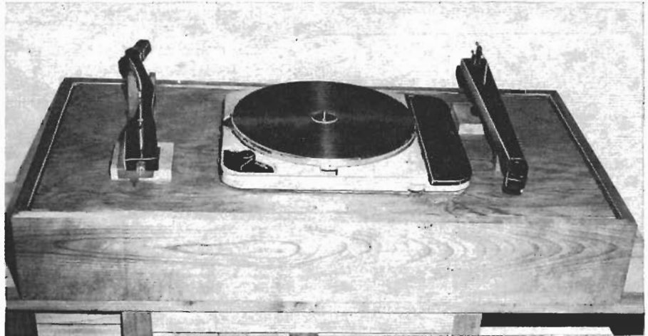
Fig. 1. Over-all view of record-player mounting arrangement described in the article. A pair of home-built tonearms complete the author's playback system.
