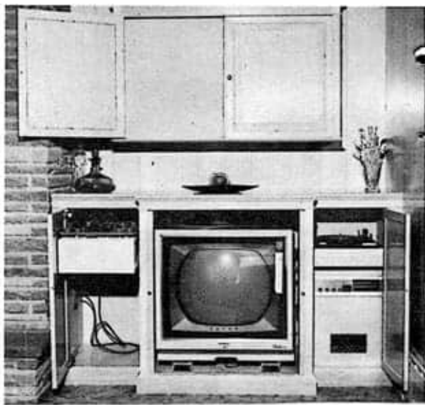
Custom cabinet holds Sargent-Raymont AM-FM tuner with stereo preamp, controls, S-R 70-watt and Acrosound 60-watt power amps, Miracord changer, Ampex 950, RCA color TV, Stephens speakers.
