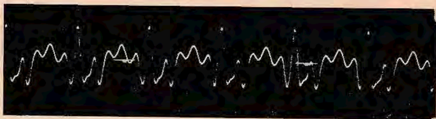
Fig. 5-5. Characteristic wave form of an oboe playing mf , at middle C. (Courtesy of Case Institute of Technology, from "The Science of Musical Sounds," by Dayton C. Miller.)
