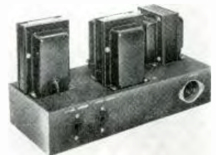
The power supply uses two big, heavy chokes.
