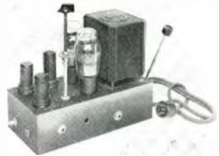
The amplifier chassis without its dust cover.
