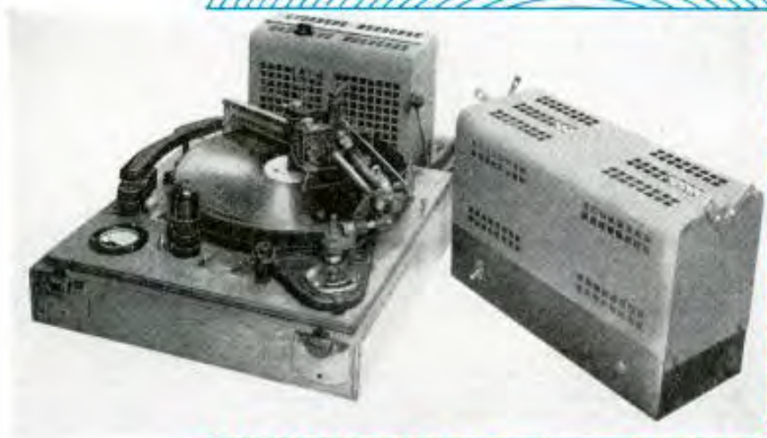
Recording components are amplifier and mechanism in case and power supply at the right.
