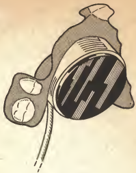
Fig. 3. An experimental denture-microphone assembly
