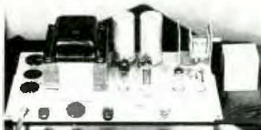
Fig. 18. Electronically regulated power supply and the preamplifier occupy the same chassis and provide interconnection between components.
