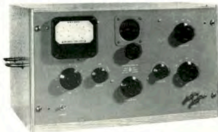
Fig. 4. Hewlett-Packard 206-A Audio Signal Generator, equipped with volume indicator and attenuators. This instrument can replace the input section of the transmission set for 50, 150 and 600 ohm circuits. A resistor and vacuum-tube voltmeter can serve as the output section.
