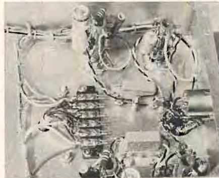
Fig. 7. Arrangement of Vector sockets for amplifier stages.
