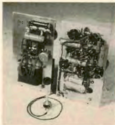
Fig. 2. Underside of the amplifier. The volume control is on an extension cable to permit flexibility in mounting.
