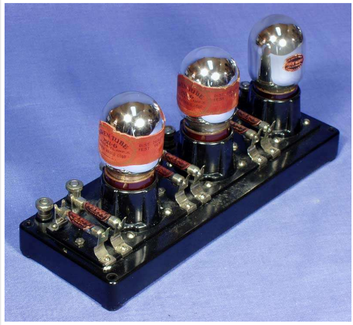
The Daven RC coupled amplifier. From the collection of Ernie Hite, Photo. Charlotte ARC
