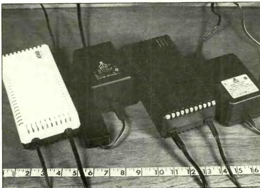
Fig. 1. Pictured here are the four major configurations of power supplies supplied with Atari XL computers arranged from Type I through Type IV left to right.
