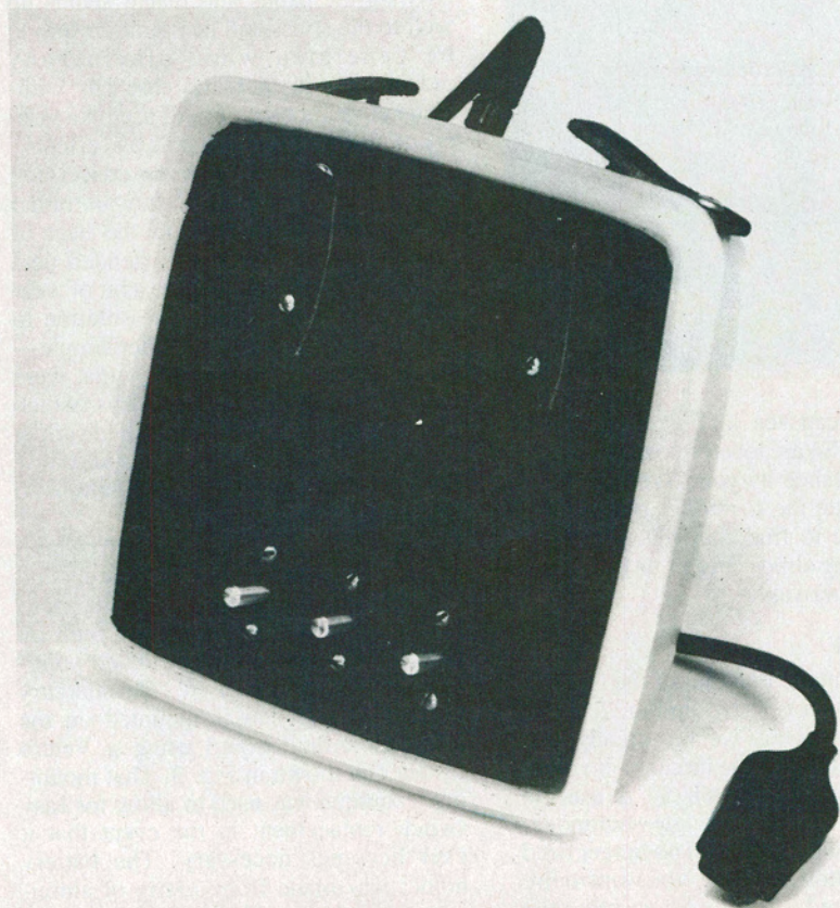
A SANDWICH BOX covered with wood-grained paper makes an inexpensive case.
