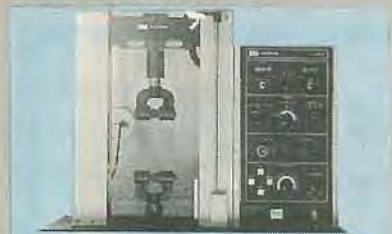
TENSILE TESTER used for measuring elongation and breaking strength.
