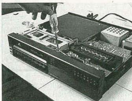
FIG. 2—THE CASSETTE CARRIAGE assembly is usually secured to the VCR chassis by four Phillips-head screws.
