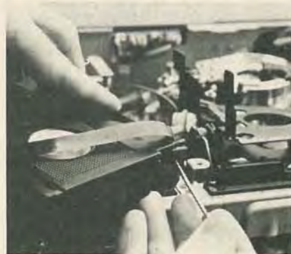
FIG. 4—WITH THE CASSETTE CLEAR, a small-tipped object such as a pencil may be used to unlatch the tape cover.
