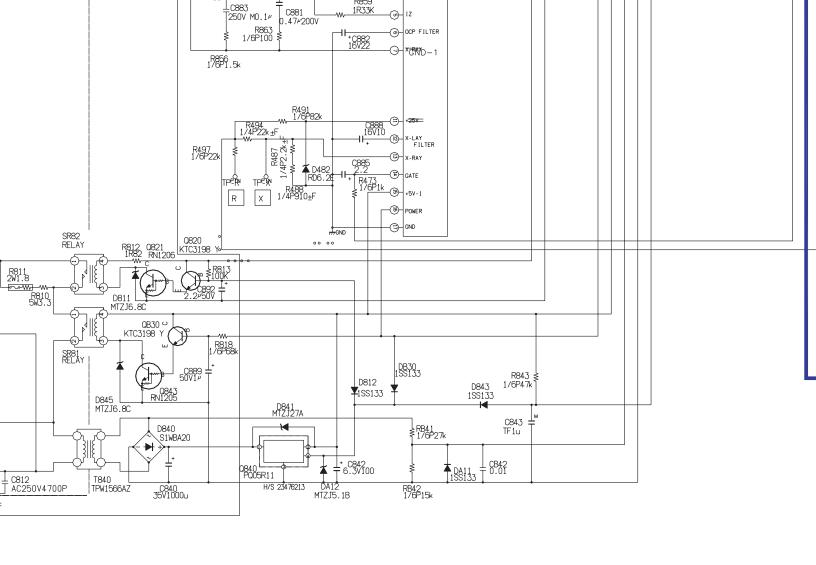
2.CAPACITOR Unless otherwise noted in schematic.aii capacitor valuee less than 1 are expressed in 4F, and the values more than 1 in pf.
